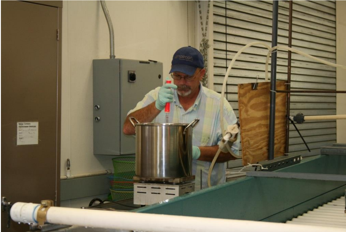
Mixing the test substance in water at 50 C. The metal pot is on a heated stir pad.
