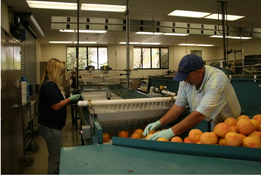
Fruit being feed onto rollers going under drench applicator
