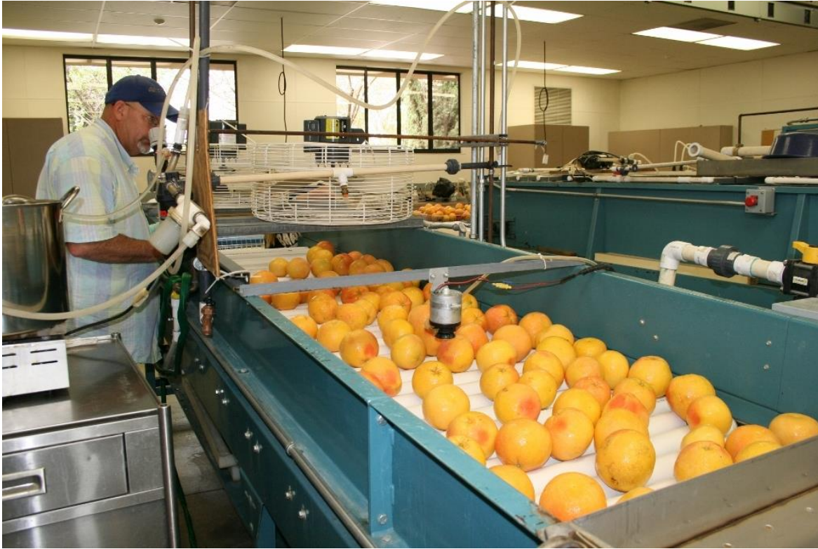
Fruit running under CDA on PVC rollers
