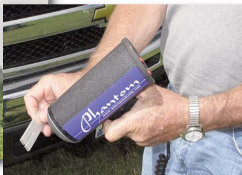
Radar gun is calibrated to 55 mph. using a tuning fork. Photo by Satoru Miyazaki
